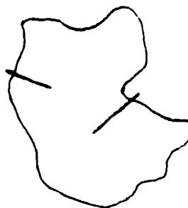
Fiber protrusion <0.5 micrometer
